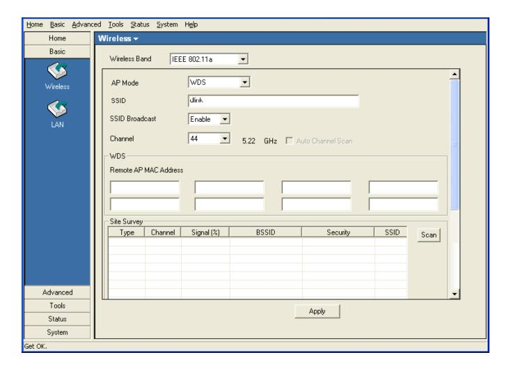
**WDS:** A Wireless Distribution System that interconnects so called Basic Service Sets (BSS). It bridges two or more wired networks together over wireless. The AP wirelessly connects multiple networks without functioning as a wireless AP.
