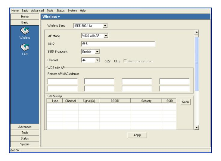
**WDS with AP:** Wireless Distribution System with Access Points. APs in a network are wirelessly wired together and connected via a Distribution System. The AP wirelessly connects multiple networks, while still functioning as a wireless AP.
