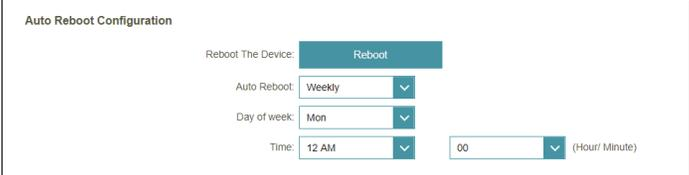
The screenshot shows the 'Auto Reboot Configuration' interface. It features a 'Reboot The Device:' section with a teal 'Reboot' button. Below this, there are three dropdown menus: 'Auto Reboot' set to 'Weekly', 'Day of week' set to 'Mon', and 'Time' set to '12 AM'. To the right of the 'Time' dropdown is a text input field containing '00' and a '(Hour/ Minute)' label.
