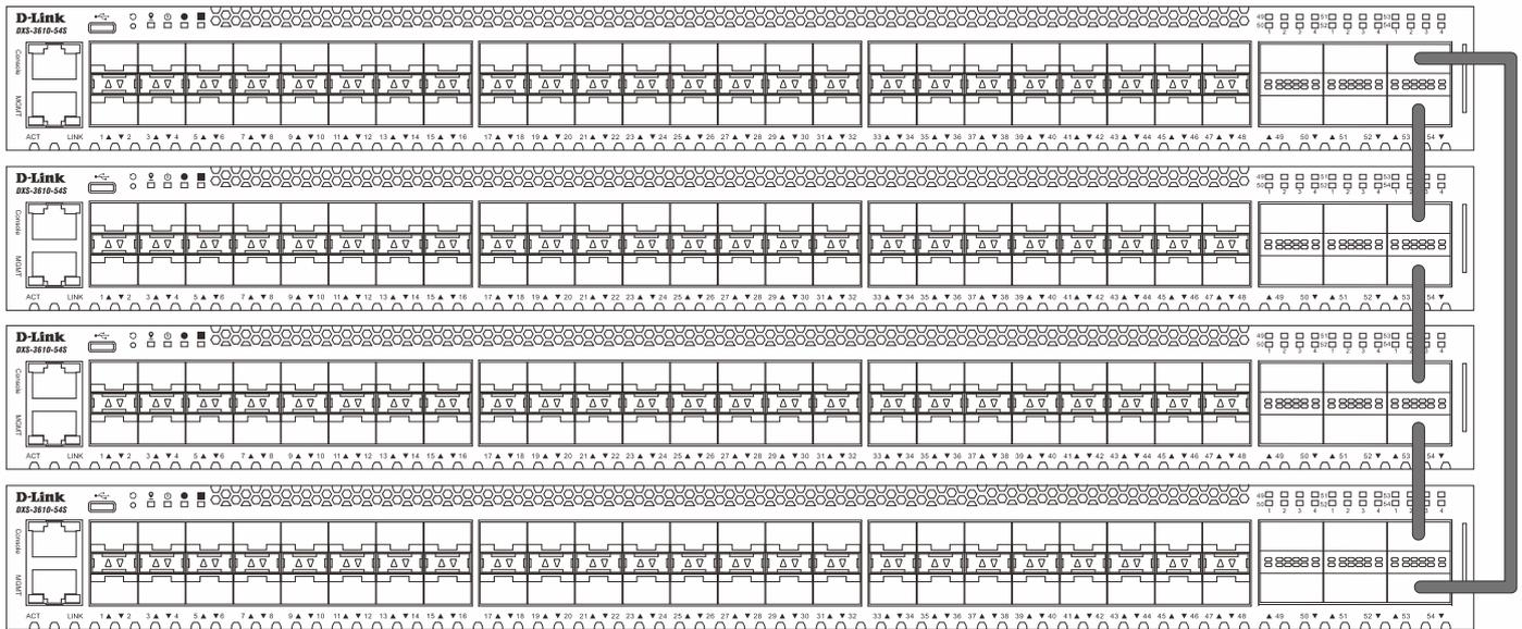
**Figure 4-2 Duplex Ring Stacking Topology**
