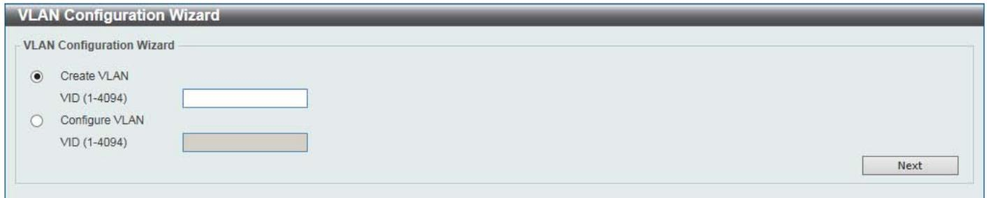
**Figure 5-9 VLAN Configuration Wizard(Select VLAN) Window**
