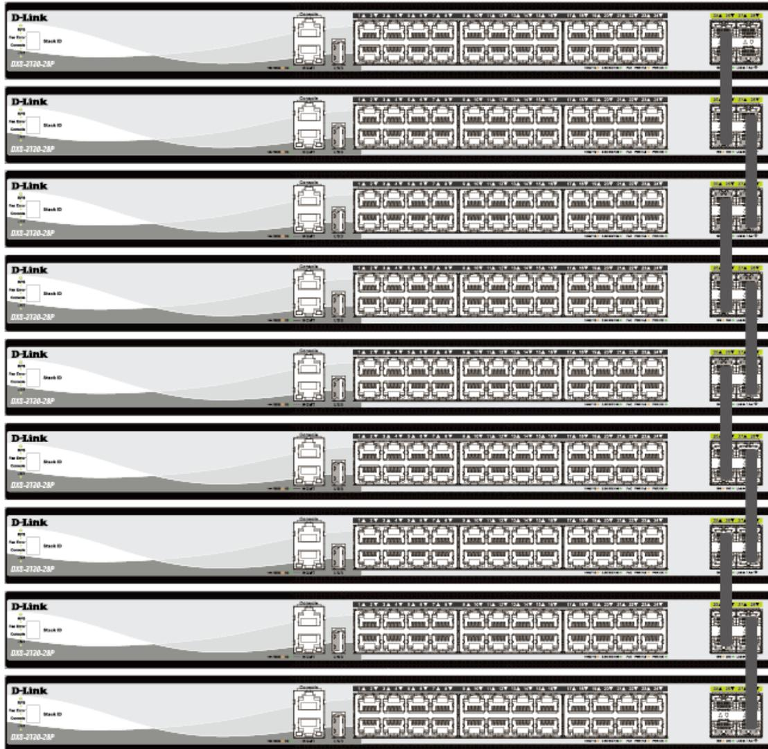
Figure 0-3 Duplex Chain stacking topology (SFP28 ports)
