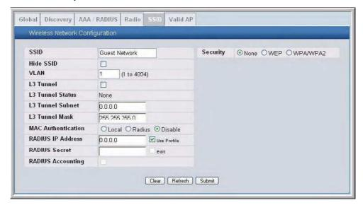
1. **VLAN Forwarding mode** – The SSID of VAP is configured to associate with a VLAN ID. When a wireless client connects to the VAP, the AP tags the client's traffic with the VLAN ID you configured. By default, all networks use VLAN 1, which is untagged.
