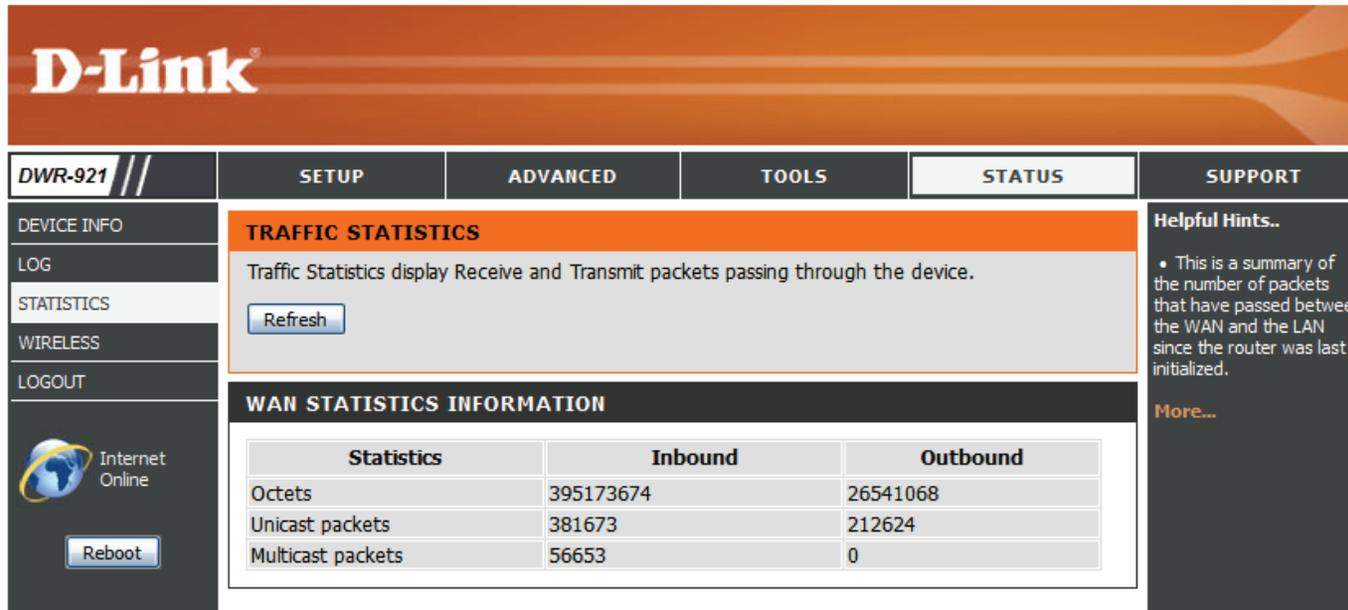
The screenshot shows the D-Link web interface for the DWR-921 router. The top navigation bar includes tabs for SETUP, ADVANCED, TOOLS, STATUS, and SUPPORT. The left sidebar contains links for DEVICE INFO, LOG, STATISTICS (highlighted), WIRELESS, and LOGOUT, along with an Internet Online status indicator and a Reboot button. The main content area is divided into two sections: TRAFFIC STATISTICS and WAN STATISTICS INFORMATION.
