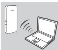
1. Power on the DWR-720 and connect your device to the dlink\_DWR-720\_xxxx wireless network, where xxxx represents the last four digits of the DWR-720's MAC address. This wireless network name as well as the password is printed on the label under the battery.
