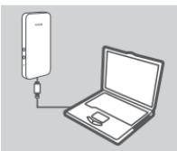
1. Power on the DWR-720 and connect it to your PC using the supplied Micro USB cable.
