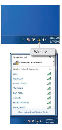
Highlight the wireless network (SSID) you would like to connect to and click the **Connect** button.
