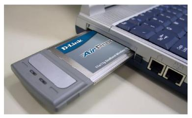
**C.** Gently insert the DWL-AG660 into the Cardbus slot in your laptop computer (as shown.)
