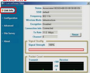
**SSID:** Service Set Identifier is a name that identifies a wireless network. Access points and wireless devices attempting to connect to a specific WLAN (Wireless Local Area Network) must use the same SSID. The default setting is **default**.
