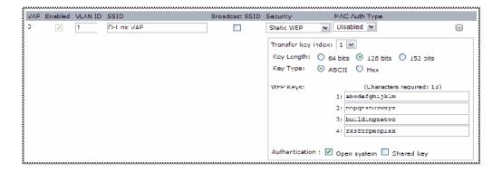
The administrator must then set all wireless client stations to use WEP and provide each client with one of the slot/key combinations defined on the AP.
