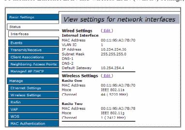
This page displays the current settings of the Unified Access Point. It displays the **Wired Settings** and the **Wireless Settings**.
