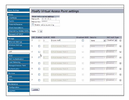
VAP 0 through VAP 7 are listed in rows, and the column headings contain the configuration options, which are described in "Configuring Virtual Access Points" on page 62. The drop-down menu in the Security column contains the following security mode options:
