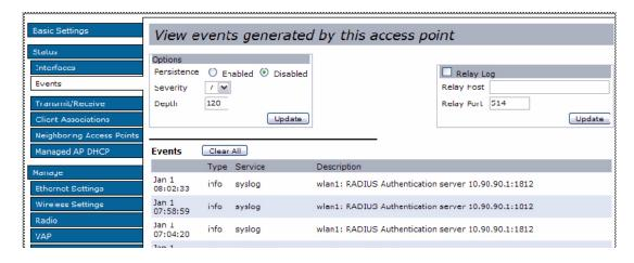
From the **Events** page, you can view the most recent events generated by this access point and configure logging settings. You can enable and configure persistent logging to write system event logs to non-volatile memory so that the events are not erased when the system reboots. This page also gives you the option of enabling a remote "log relay host" to capture all system events and errors in a Kernel Log.
