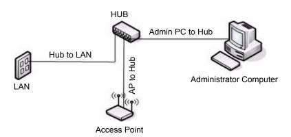
The hub or switch you use must permit broadcast signals from the access point to reach all other devices on the network.
