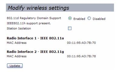
NOTE: For the DWL-8500AP, radio interface settings apply to both Radio Interface 1 and Radio Interface 2.
