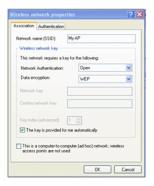
Use this dialog for configuring all the different types of client security described in the following sections. Make sure that the wireless network properties you configure are for the network name (SSID) for the network you want to reach on the wireless client.
