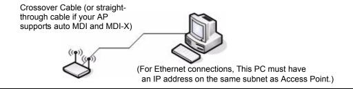
For initial configuration with a direct Ethernet connection and no DHCP server, be sure to set your PC to a static IP address in the same subnet as the default IP address on the access point. (The default IP address for the access point is 10.90.90.91.)
