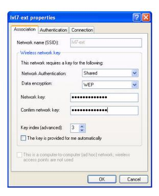
Additional wireless clients also need to have one of the WEP keys defined on the AP. The administrator can assign the same WEP key that the first client has, or the administrator can give the second station a different WEP key (key 2, for example) so that the two stations cannot decrypt each other's transmissions.
