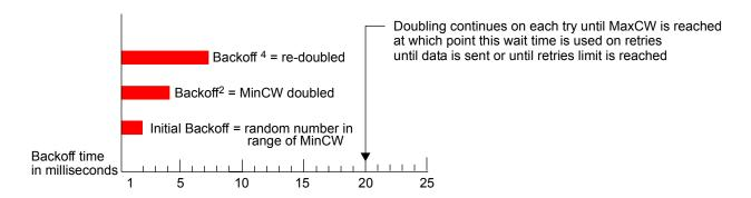
The random backoff used by the access point is a configurable parameter. To describe the random delay, a "Minimum Contention Window" (MinCW) and a "Maximum Contention Window" (MaxCW) is defined.
