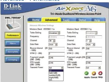
Wireless Band: Select 802.11a (up to 72 Mbps speed in turbo mode in the 5GHz range) or 802.11g (up to 54 Mbps\* speed with AirPlus adapters.)
