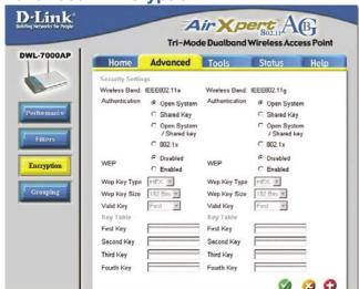
802.1x - is the first line of defense against network intrusion. In the authentication process the Radius Server verifies the identity of the client attempting to connect to the network. Unfamiliar clients will be denied access. **EAP**(Extensible Authentication Protocol) is available through the Windows XP Operating System. You will need to use the same type of EAP protocol on all the devices in your network when using the 802.1x feature.
