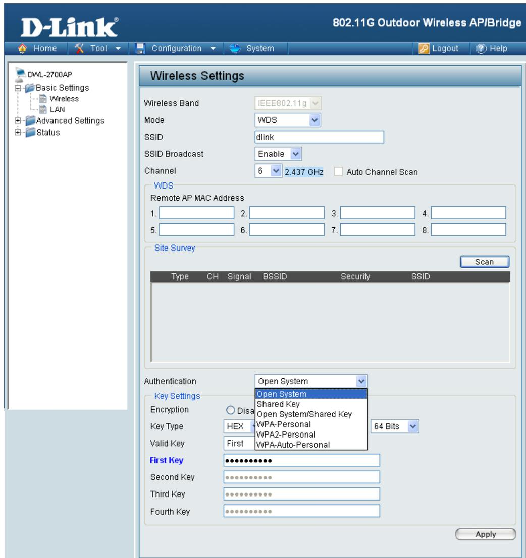
In WDS, the **DWL-2700AP** wirelessly connects multiple networks, without functioning as a wireless AP.
