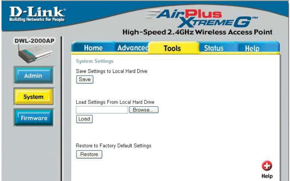
The current system settings can be saved as a file onto the local hard drive. The saved file or any other saved setting file can be loaded back on the DWL-2000AP. To reload a system settings file, click on **Browse** to browse the local hard drive and locate the system file to be used. You may also reset the *Wireless Access Point* back to factory settings by clicking on **Restore**.
