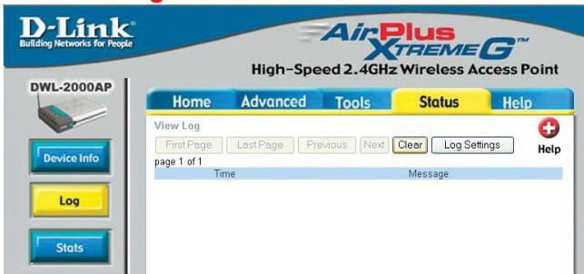
The Log keeps a running log of events and activities occurring on the Access Point. If the device is rebooted, the logs are automatically cleared. You may save the log files under Log Settings.
