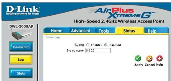
When you click on **Log Settings** in the previous window, the window at left appears. Select **Enabled** to save the log. In the **Syslog Server** field, input the IP Address of the computer on the network to which you wish to save the log settings. Click **Apply** to save the changes.
