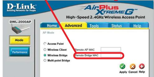
When using the DWL-2000AP in **Wireless Bridge** mode, you will enter the MAC address of the Remote Bridge.
