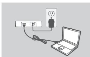
3. Plug the Type A connector end of the included USB cable into an available USB port on your computer.
