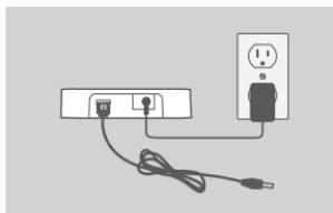
2. Plug the smaller (Mini-B USB) end of the included USB cable into the back of the DUB-H4.
