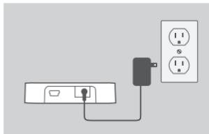
1. Plug the power adapter into the receptor located on the back of the DUB-H4. Plug the other end into a wall outlet. The LED on the DUB-H4 will turn green to indicate that the hub is receiving power.
