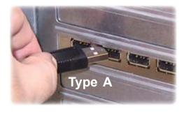
**D.** Your computer will automatically detect and install the DUB-H4. You may now connect USB 2.0 or USB 1.1 devices to an available USB port on the front of the DUB-H4.
