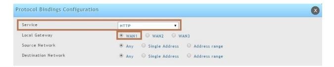
Please notice that when we run traffic (FTP,SSH,telnet etc.) which are not configured in protocol binding page, then traffic can go through WAN1 or WAN2 as wan mode is in load balancing round robin. When services such as (HTTP/DNS/HTTPS) is requested, the traffic is sent through WAN1.
