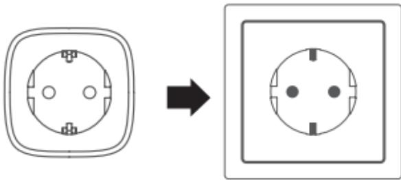
Plug the Mini Wi-Fi Smart Plug into a power outlet. Wait until the LED on the front changes from red to flashing amber.
