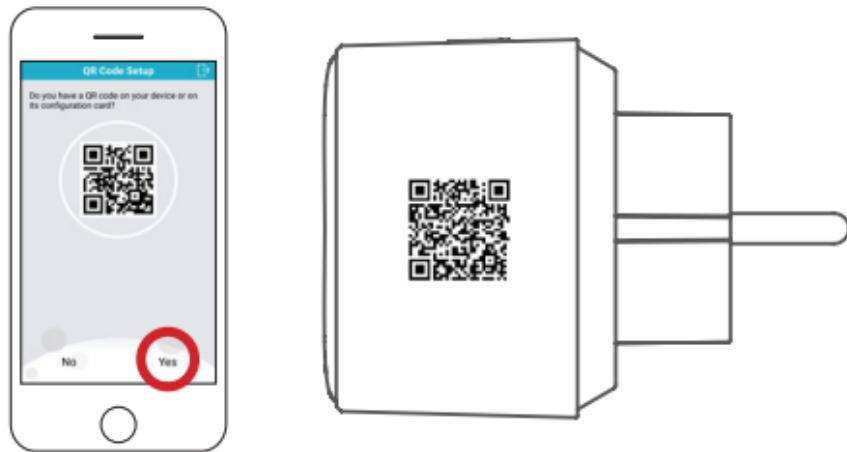
When asked to scan a Setup Code, it will be located on the right side of your Mini Wi-Fi Smart Plug.
