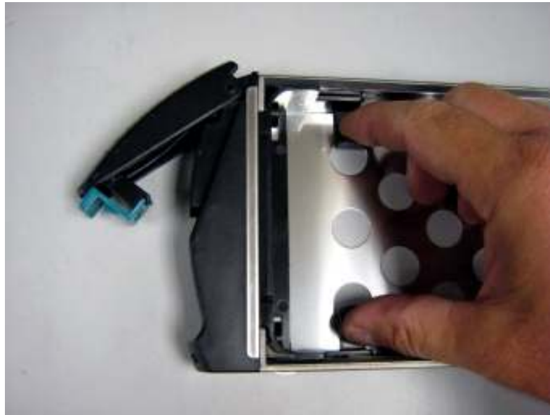
Figure D-9 Removing the Plastic Air Dam Piece
