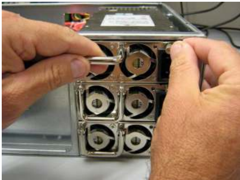
Figure D-20 Push the Locking Lever to the Left and Pull Handle
