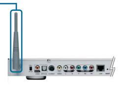
Note: You may have an Ethernet cable plugged into the unit and have the wireless antenna connected. Neither will interfere with the other, but only one network can be accessed at a time (wired or wireless). The network connection type is selected in the Setup Wizard and can be changed by going to the Setup Menu. To access the Setup Menu, press the SETUP button on the remote control.
