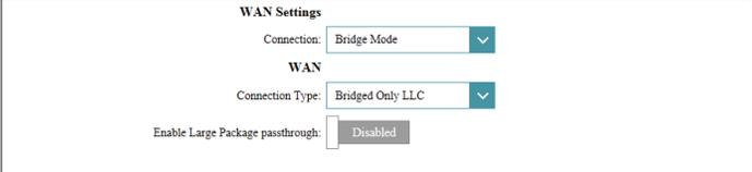
The screenshot shows the WAN Settings configuration interface. It includes a 'WAN Settings' section with a 'Connection' dropdown menu set to 'Bridge Mode'. Below this is a 'WAN' section with a 'Connection Type' dropdown menu set to 'Bridged Only LLC'. At the bottom, there is a checkbox for 'Enable Large Package passthrough' which is currently disabled.
