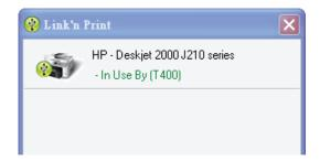
3. Move the cursor to In Use By (Owner) and click on Disconnect to virtually disconnect the USB device.
