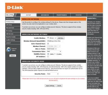
Wireless Here, you can select between None, WEP, WPA-Personal, and WPA-**Security Enterprise.** Refer to the following pages for details on configuring the Mode: different security modes. Please note that using WEP encryption will limit wireless use to 802.11g/b only, as it is incompatible with 802.11n.
