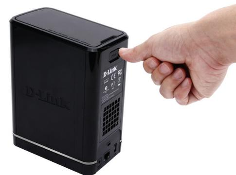
3. Once the faceplate is unlatched, remove it to expose the hard drive bays.
