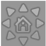
**PTZ Control:** You can control the camera view by utilizing the PTZ (pan, tilt, and zoom) camera control panel to adjust the camera angle. This function is only available with cameras that support the PTZ function.
