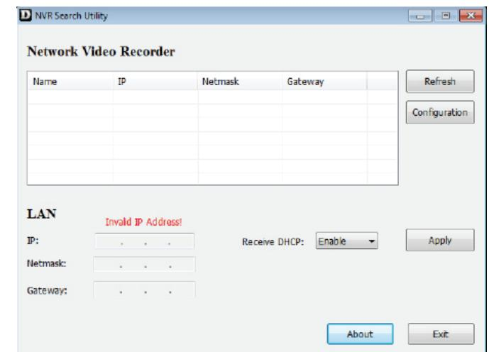
Select a device from the list and click **Configuration**. This will launch the computer's default web browser and direct it to the IP address listed for the device. Make sure the browser is not configured to use a proxy server.
