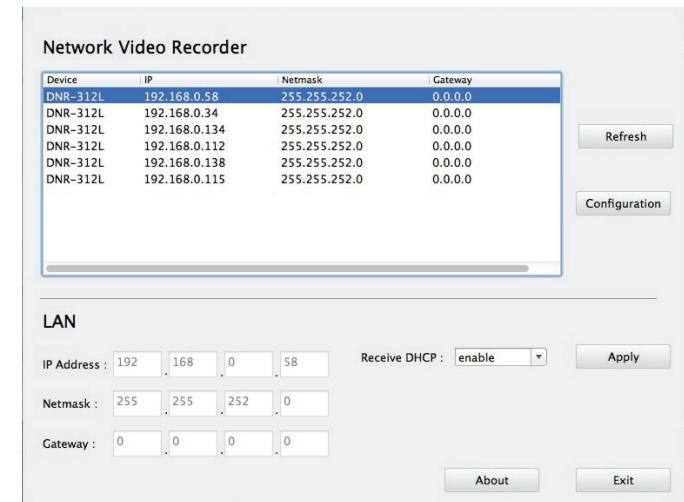
Select the device from the list and click **Configuration**. This will launch the computer's default web browser and direct it to the IP address listed for the device. Make sure the browser is not configured to use a proxy server.
