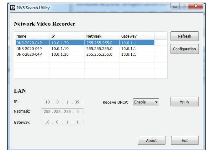
Select a device from the list and click **Configuration**. This will launch the computer's default web browser and direct it to the IP address listed for the device.
