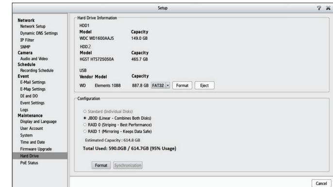
**HDD format Standard (Individual Disks):** Only supports one hard drive to create the volume.
