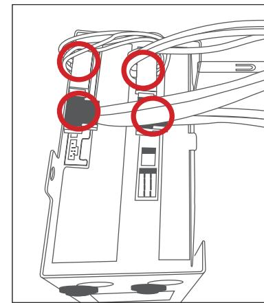
5. Re-attach the drive bay bracket to the device enclosure by sliding the tabs into the holes and using the screws provided to secure it.
