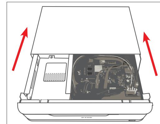
3. Detach the HDD bay bracket, then insert one or two 3.5" SATA hard drives into the drive bays and use the provided screws to secure the drives in the bracket.
