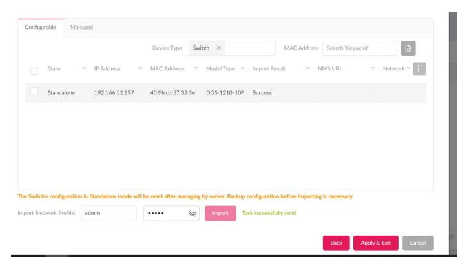
10. Click Re-Discovery button and Managed tab display the switch(example switch: DGS-1210-10P) is managed, then click "Apply & Exit"
