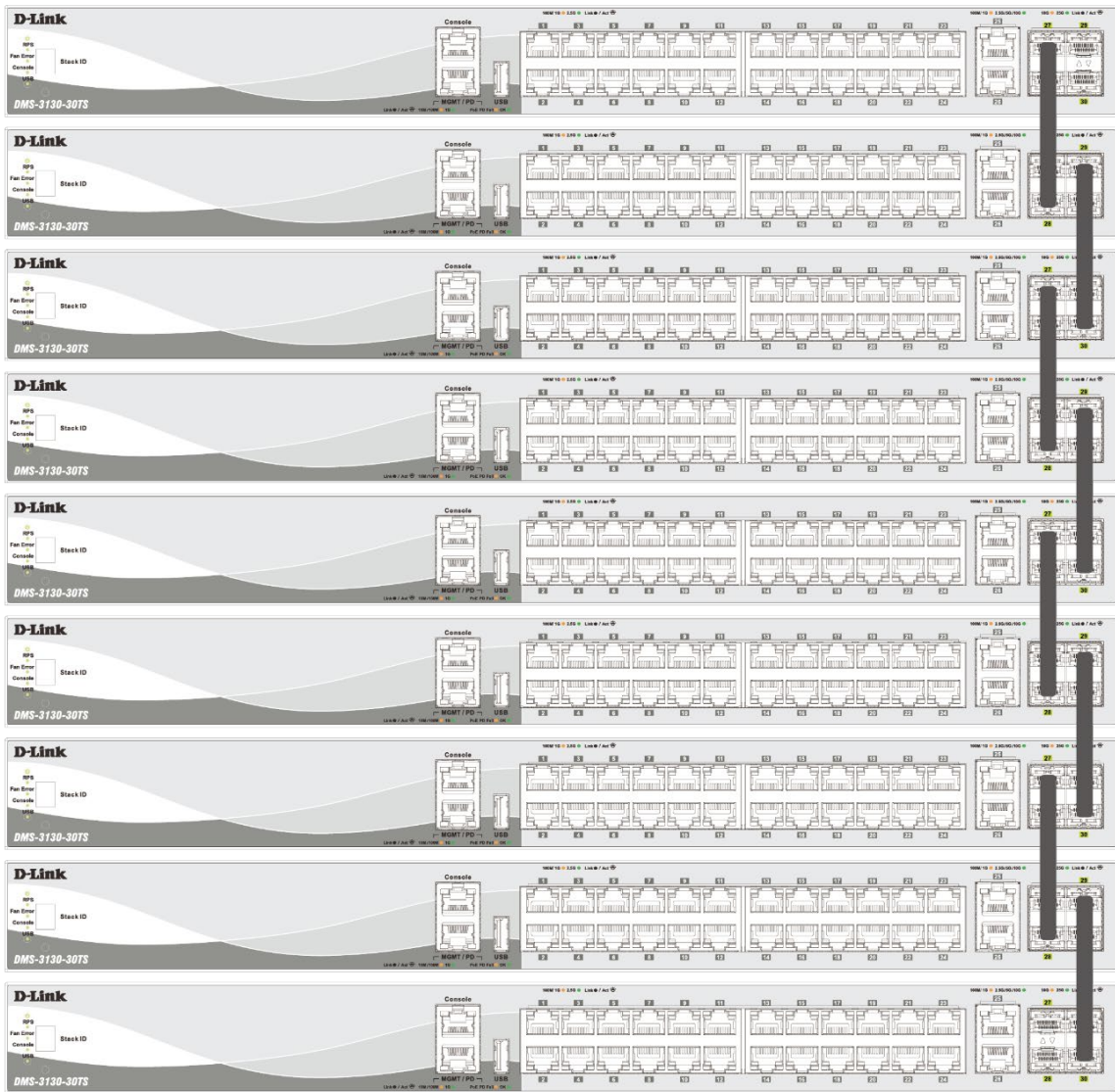
Figure 4-4 4-Port Duplex Chain stacking topology (SFP28 ports)
