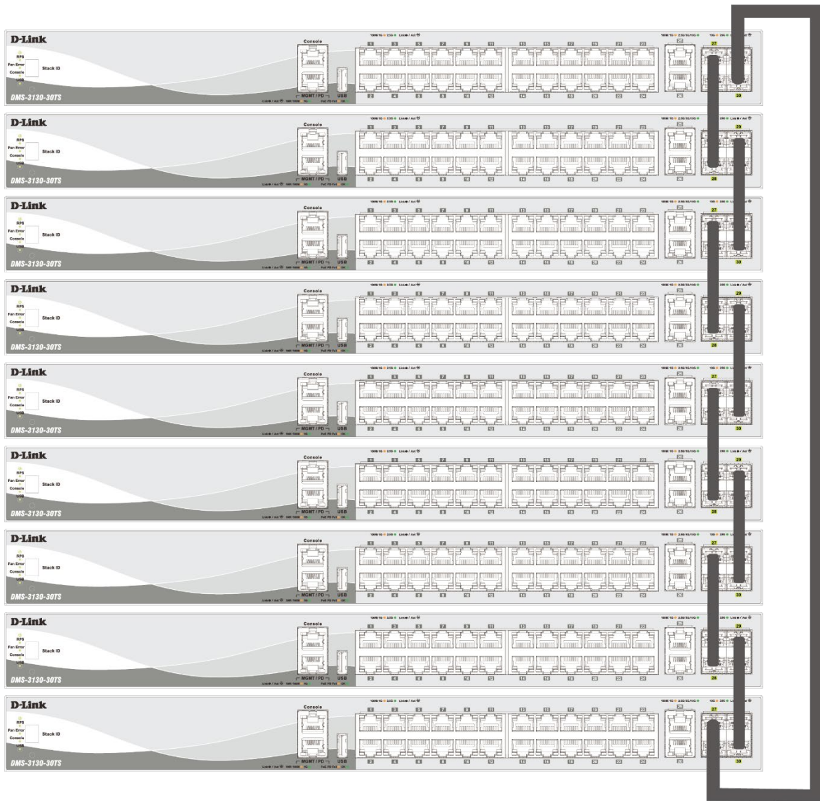
Figure 4-6 4-port Duplex Ring stacking topology (SFP28 ports)
