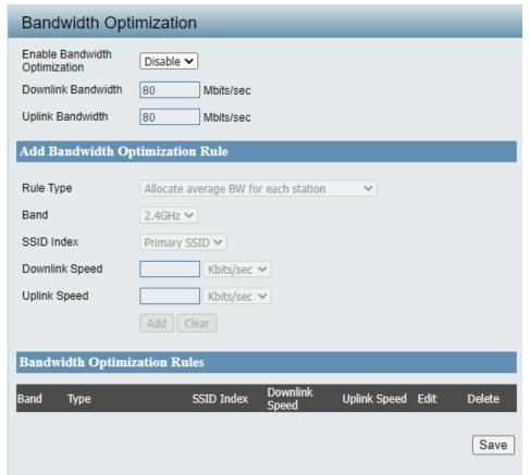
Band: Use the drop-down menu to toggle the wireless band between 2.4GHz and 5GHz.
