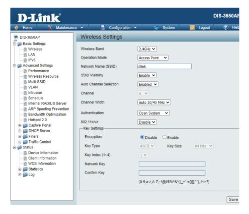
**Channel:** To change the channel, first toggle the *Auto Channel Selection* setting to **Disable**, and then use the drop-down menu to make the desired selection.
