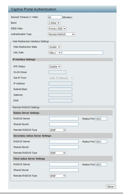
**IP Address:** Assign a static IP address that is within the IP address range of your network.
