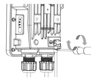
4. Tighten the grounding wire (green-and-yellow, 18AWG) to the DIS-3650AP until it is securely attached.
