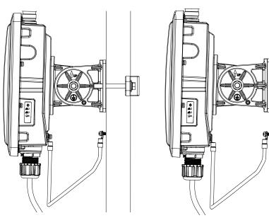
5. Attach the other end of the grounding wire to either the wall or pole mount. Ensure that the wall or pole mount is connected to an electrical ground.
