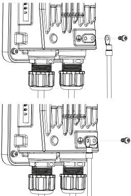
3. A grounding wire is to protect your device from lightning strikes and the buildup of static electricity. Attach the grounding wire to the DIS-3650AP using the included screw(M3.9 \* 7.8 mm).
