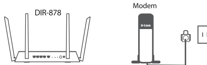
4. Use the included Ethernet cable to connect your modem to the yellow port labeled **INTERNET** on the router.
