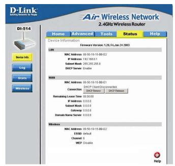
If your WAN connection is set up for **PPPoE**, a **Connect** button and **Disconnect** button will be displayed. Use **Disconnect** to drop the PPPoE connection and use **Connect** to establish the PPPoE connection.
