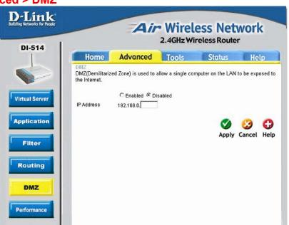
If you have a client PC that cannot run Internet applications properly from behind the DI-514, then you can set the client up to unrestricted Internet access. It allows a computer to be exposed to the Internet. This feature is useful for gaming purposes. Enter the IP address of the internal computer that will be the DMZ host. Adding a client to the DMZ (Demilitarized Zone) may expose your local network to a variety of security risks, so only use this option as a last resort.
