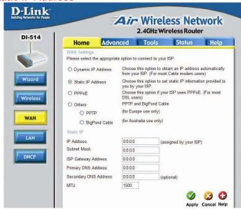
Choose Static IP Address if all WAN IP information is provided to you by your ISP. You will need to enter in the IP address, subnet mask, gateway address, and DNS address(es) provided to you by your ISP. Each IP address entered in the fields must be in the appropriate IP form, which are four IP octets separated by a dot (x.x.x.x). The Router will not accept the IP address if it is not in this format.
