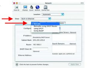
Input the **Static IP Address**, the **Subnet Mask** and the **Router IP Address** in the appropriate fields.
