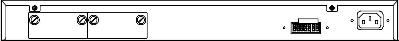
Figure 2- 7. Rear panel view of DGS-3426
