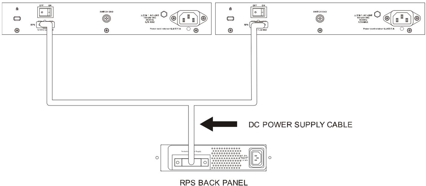
Figure 3-10 Connecting the DPS-200A to two Switches
