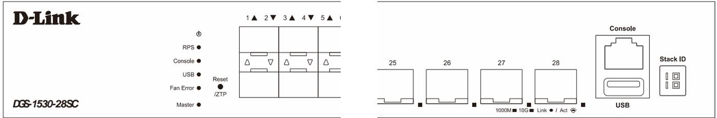
Figure 2-16 DGS-1530-28SC Front Panel (LED Indicators)
