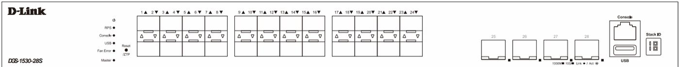
Figure 2-7 DGS-1530-28S Front Panel
