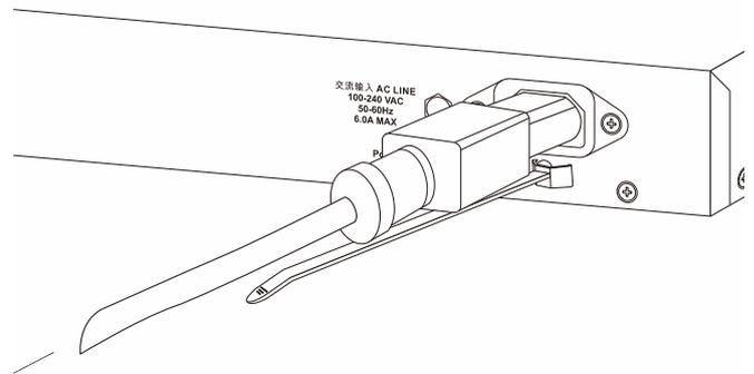
Figure 3-6 Connect the power cord to the Switch
