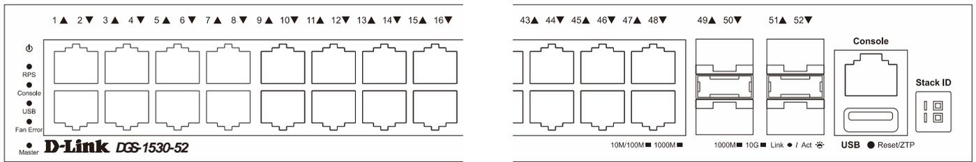
Figure 2-12 DGS-1530-52 Front Panel (LED Indicators)
