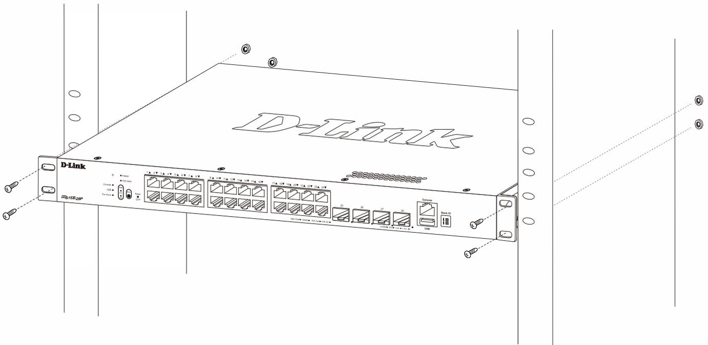
Figure 3-3 Installing the Switch in a Rack
