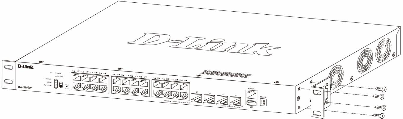
Figure 3-2 Attaching the rack-mounting brackets
