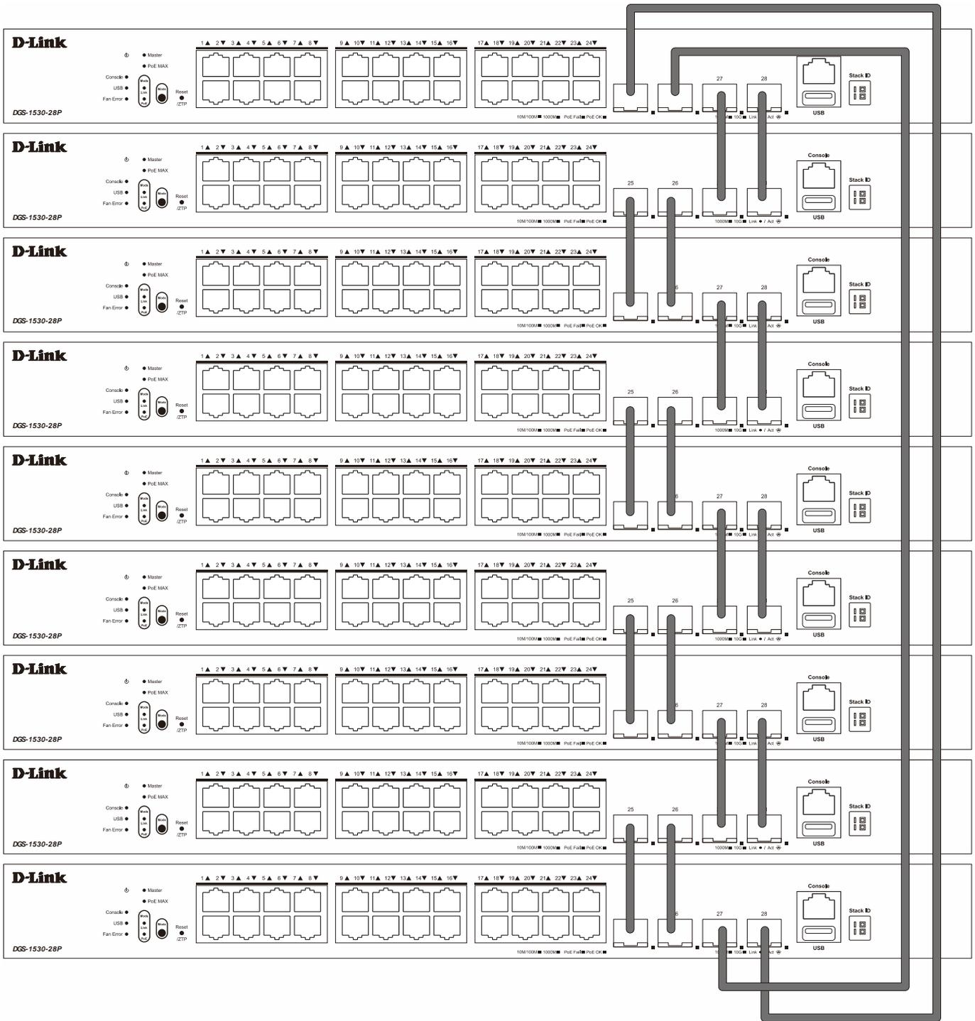
**Figure 4-2 Duplex Ring Stacking Topology**
