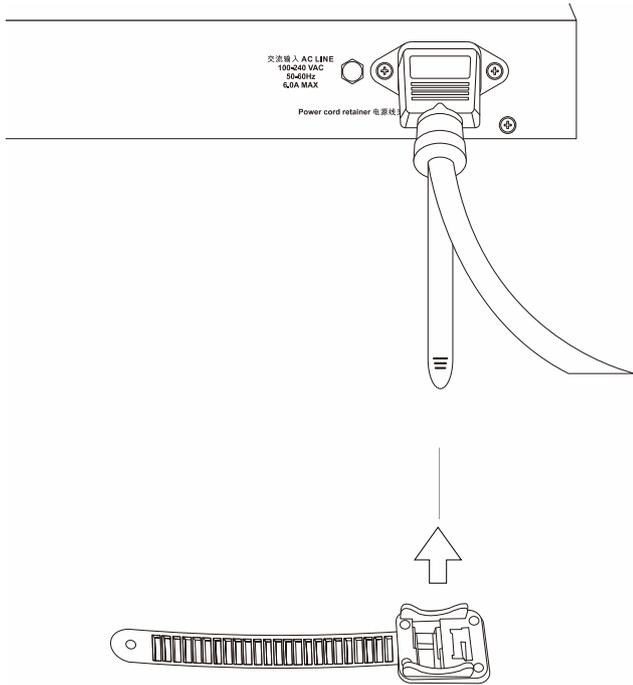
Figure 3-7 Slide the Retainer through the Tie Wrap
