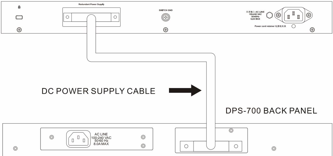
Figure 3-12 Connecting the DPS-700 to the Switch
