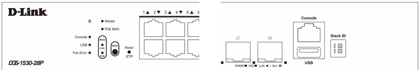
Figure 2-13 DGS-1530-28P Front Panel (LED Indicators)
