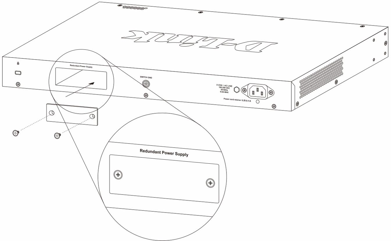
**Figure 3-13** Reinstalling the RPS port cover
