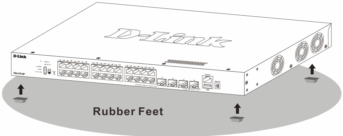
Figure 3-1 Attaching rubber feet to the Switch
