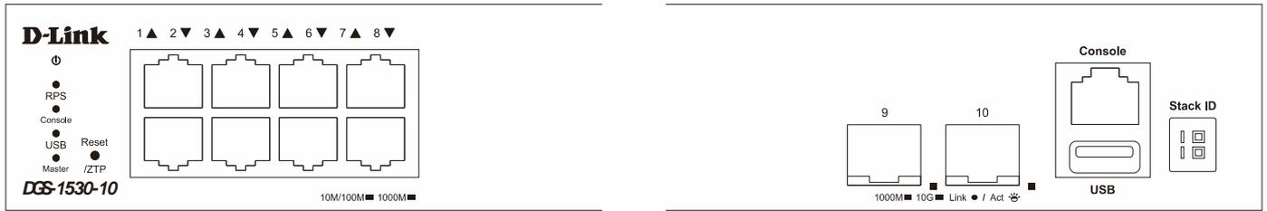
Figure 2-9 DGS-1530-10 Front Panel (LED Indicators)
