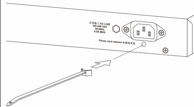
Figure 3-5 Insert Tie Wrap into the Switch
