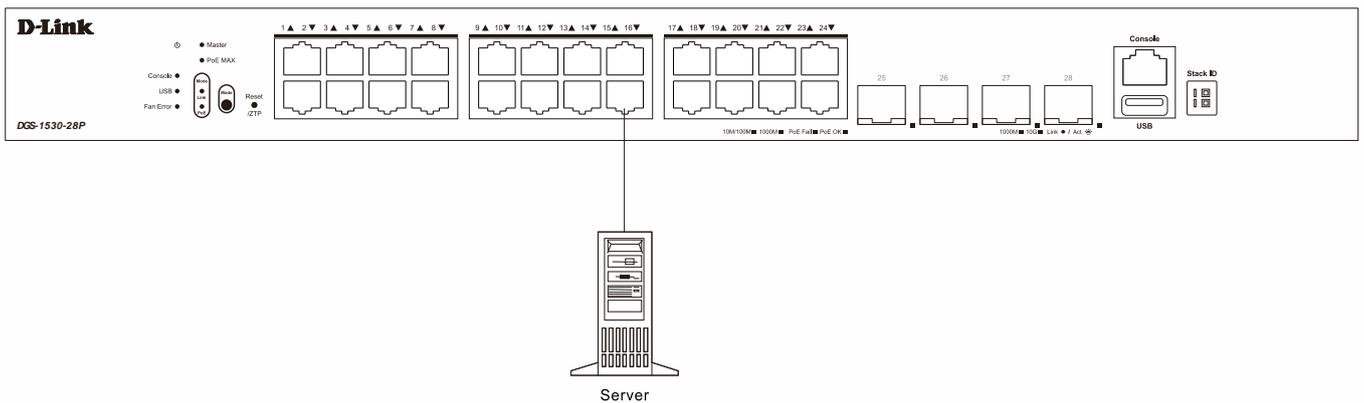
Figure 4-5 Switch to End Node (Server)
