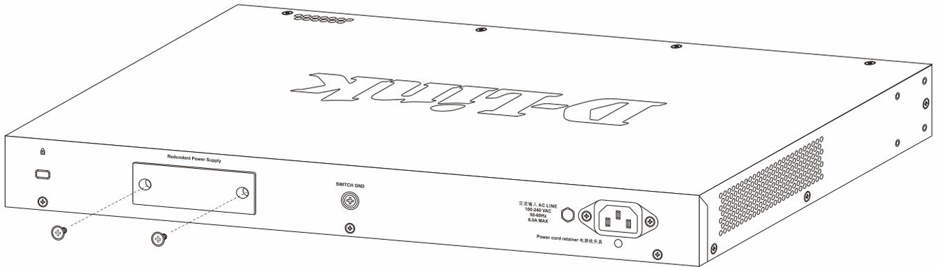
Figure 3-11 Removing the RPS port cover
