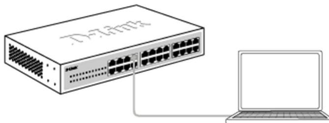
Figure 4-1 Connecting to a DGS-1100 MP/MPP Series switch
