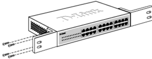
Figure 3-2 Attach the mounting brackets to the switch
