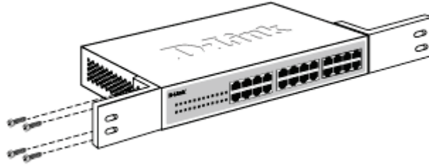
Figure 3-2 – Attach the mounting brackets to the switch
