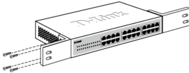
Figure 3-2 Attach the mounting brackets to the switch
