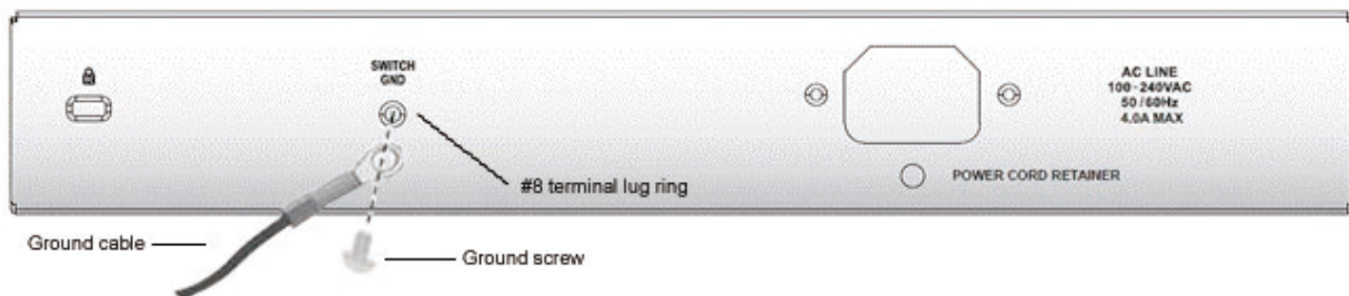
Figure 4 – Attaching a grounding cable
