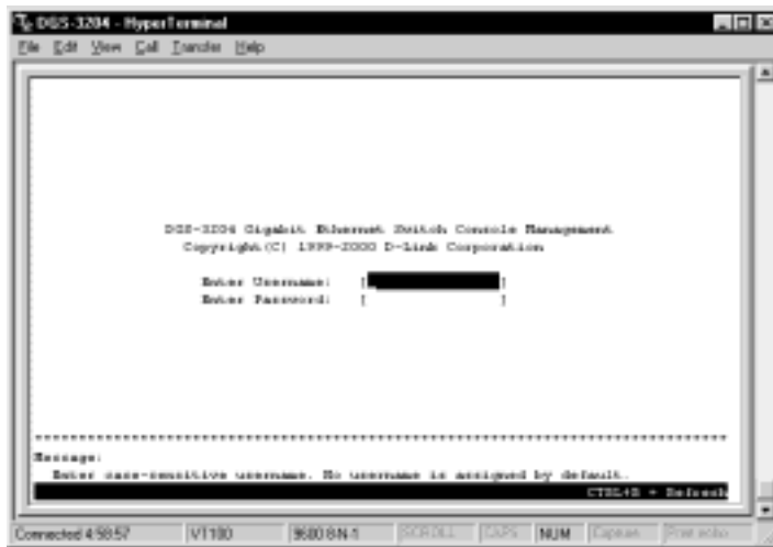
Figure 6-1. Initial Screen, first time connecting to the Switch
