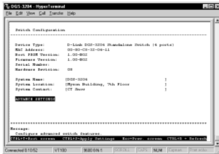
Figure 6-10. Switch Configuration screen
