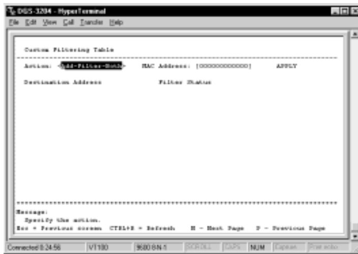
Figure 6-19. Custom Filtering Table screen
