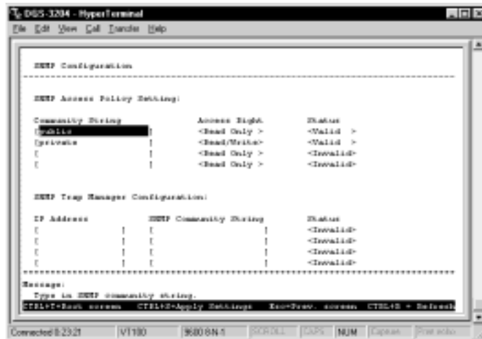
Figure 6-23. SNMP Configuration screen
