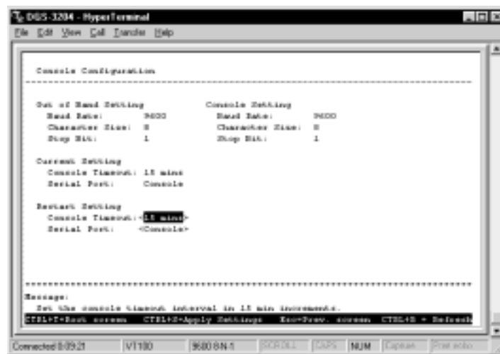
Figure 6-9. Console Configuration screen
