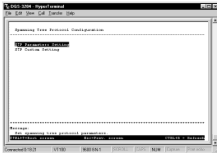
Figure 6-14. Spanning Tree Protocol Configuration menu
