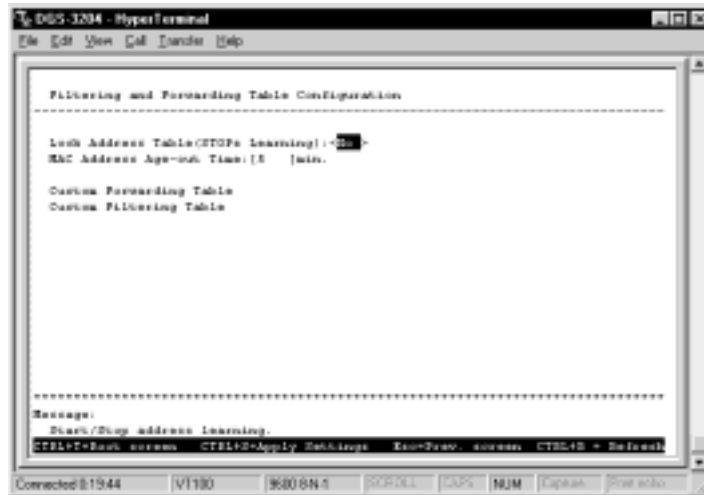
Figure 6-17. Filtering and Forwarding Table Configuration screen
