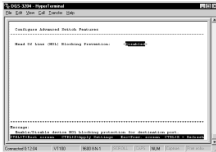
Figure 6-11. Configure Advanced Switch Features screen
