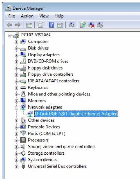
To check that the installation of the **DGE-528T** was successful, scroll down and click on **“Network Adapters.”**
