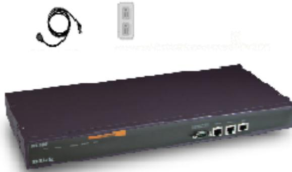
Connect the power cord to the DFL-1000 and plug it in. The **Power** indicator on the front panel will light up and then the **Status** light will begin flashing, indicating that startup has begun. After about 45 to 60 seconds the DFL-1000 will be ready for use.
