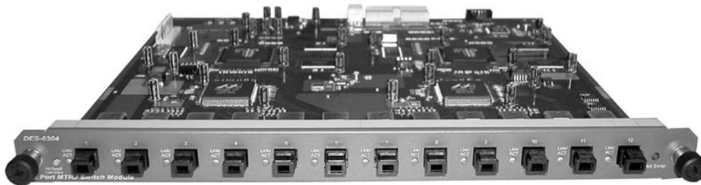
Figure 3-3. Twelve-port, 100BASE-FX (MT-RJ) module
