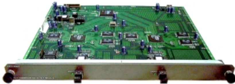
Figure 3-4. Two-port, 1000BASE-SX (MT-RJ) module
