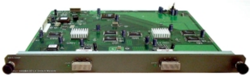
Figure 3-6. Two-port, 1000BASE-LX gigabit module
