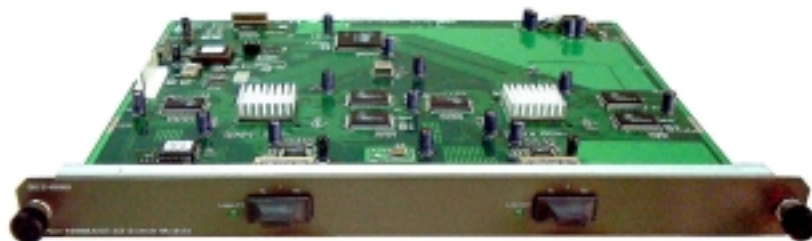
Figure 3-5. Two-port, 1000BASE-SX gigabit module
