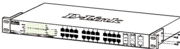
Figure 2 – Attach the mounting brackets to the Switch
