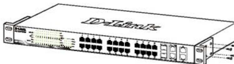
Figure 10 – Attach the mounting brackets to the Switch
