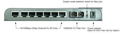
**DC Power Jack:** Power is supplied through an external AC power adapter. Since the switch does not include a power switch, plugging its power adapter into a power outlet will immediately power it on.
