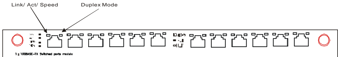
Figure 11: 16-Port 10/100-TX Module
