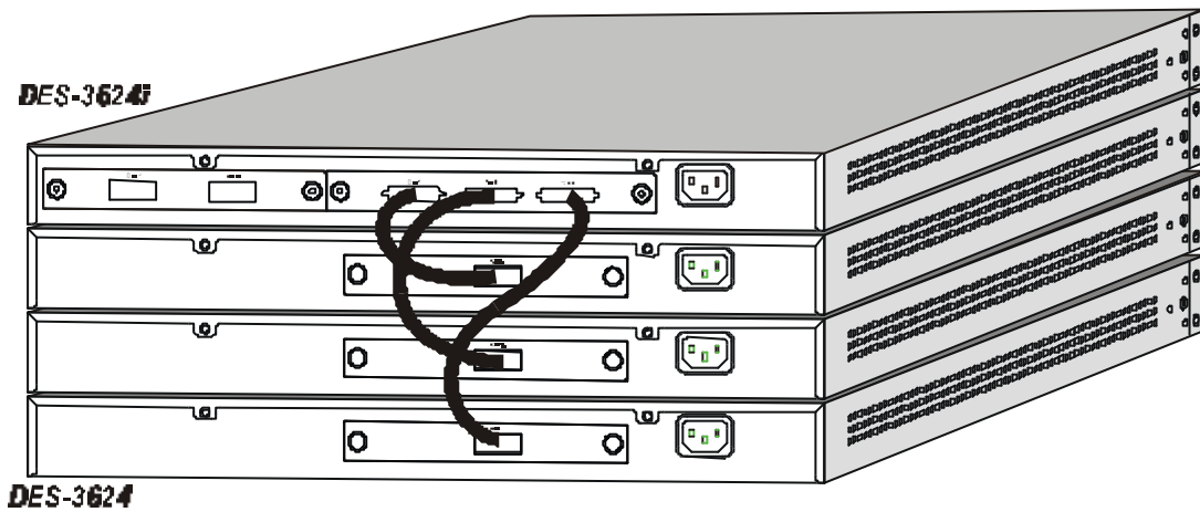
Figure 3-4. Switch stack with one master and three slaves
