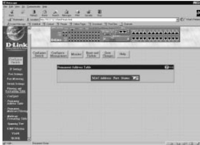
**MAC forwarding allows the Switch to permanently forward outbound traffic to specific destination MAC addresses over a specified port. You can also use this feature to restrict inbound traffic based on source MAC addresses.**
