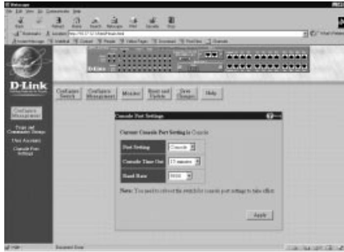
This window allows you to select the protocol for communicating through the console port, *Console* or *SLIP*, in the Port Setting field. Use SLIP for out-of-band management. You can also choose the refresh rate in the Console Time Out field (*15 minutes*, *30 minutes*, *45 minutes*, *60 minutes* or *Never*). If SLIP is being used, you may also set the Baud Rate in the last field. Click Apply and then reboot the Switch for console port settings to take effect.
