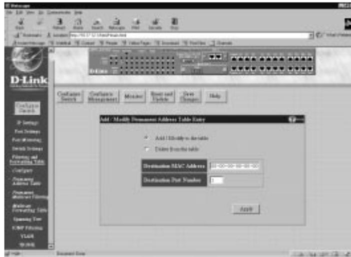
To use the MAC forwarding function, check either the **Add/Modify to the table** option button or the **Delete from the table** option button, enter the MAC address of the device to which the specified port permanently forwards traffic in the **Destination MAC Address** field, and enter the port number that permanently forwards traffic from the specified device in the **Destination Port Number** field. Then click **Apply**.
