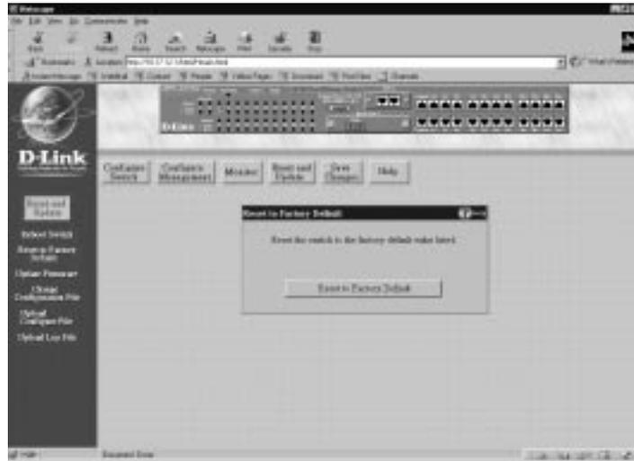
**Doing a remote reset is equivalent to turning the Switch off and on again. All parameters are returned to the values stored in EEPROM. Click the Reset to Factory Default to reset the Switch.**
