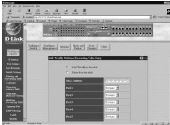
To Add/Modify to the table or Delete from the table, check the desired option button, enter the MAC address in the MAC Address field, select *Forward* or *Block* for each port, deciding whether that port transmits or blocks traffic for the specified multicast group. Click **Apply** to let the changes take effect.
