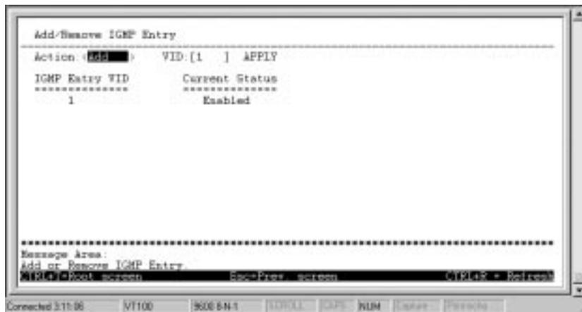
The above window is used to specify an agent to interface between IGMP and VLAN. The agents are assigned to a VLAN and allow IGMP query and report packets to be present on the given VLAN. Only 12 agents can exist on the switch at any one time.
