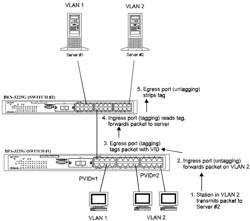
**In the above example, step 4 is the key element. Because the packet has 802.1Q VLAN data encoded in it's header, the ingress port can make VLAN-based decisions about its delivery - whether server #2 is attached to a port that is a member of VLAN 2 and thus should the packet be delivered, the queuing priority to give to the packet, etc. It can also perform these functions for VLAN 1 packets as well, and in fact, for any tagged packet it receives regardless of the VLAN number.**
