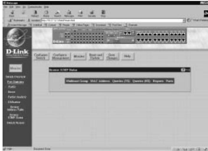
**This window allows you to display Multicast Group, MAC Address, Queries (TX), Queries (RX), Reports, and Ports for IGMP Snooping in a table format.**
