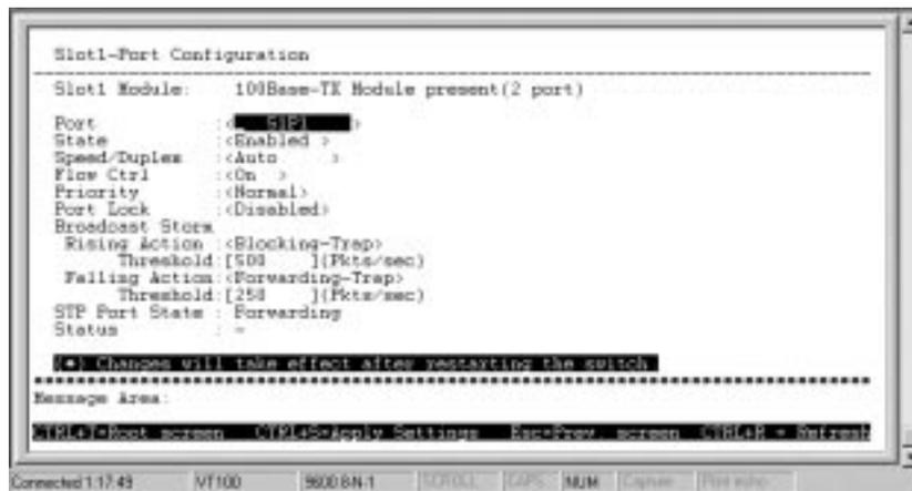
Figure 6-13. Slot1-Port Configuration screen
