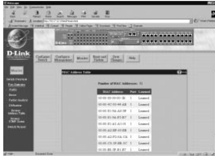
**The Switch allows you to display a table containing MAC addresses, ports, and respective learned statuses. Clicking the Next Page hyperlink at the bottom of the screen will allow you to display the complete MAC Address Table.**
