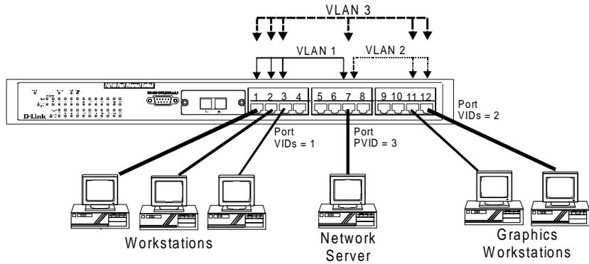
In the above example, there are three different VLANs and each port can transmit packets on one of them according to their Port VLAN ID (PVID) number. However, a port can receive packets on all VLANs (VID) that it belongs to. The assignments are as follows:
