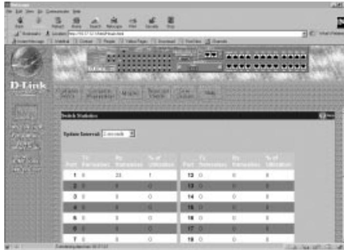
The screenshot shows the D-Link web-based network management interface. The 'Link & Statistics' page is displayed, showing a table of port statistics. The 'Update Interval' is set to 2 seconds. The table has columns for Port, TX frames/sec, RX frames/sec, and % of Utilization. The data is as follows:
