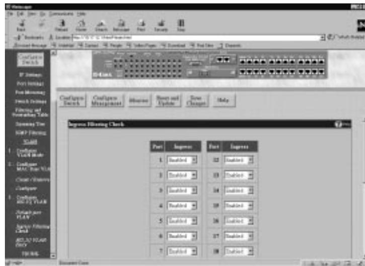
**Use this window to enable or disable the ingress filtering check for each desired port. Ingress filtering means that a receiving port will check to see if it is a member of the VLAN ID in the packet before forwarding the packet. Click Apply to let the settings take effect.**
