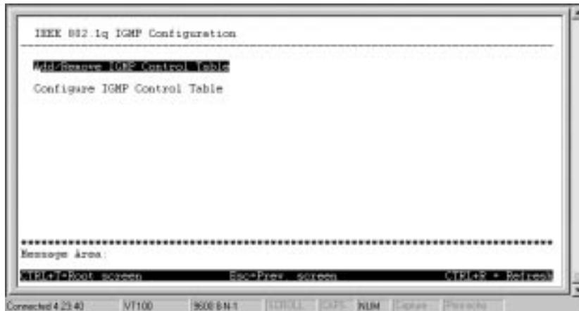
Choosing *Add/Remove IGMP Entry* allows you to define up to 12 VLANs on the switch which can send and receive IGMP packets. Choosing *Configure IGMP Control Table* allows you to enable/disable these agents and set aging timers for them. Both windows are shown below:
