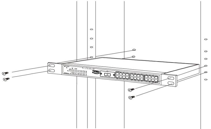
Figure 2-2B. Installing the switch on an equipment rack
