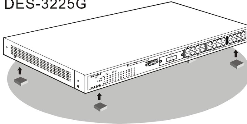
Figure 2-1. Installing rubber feet for desktop installation
