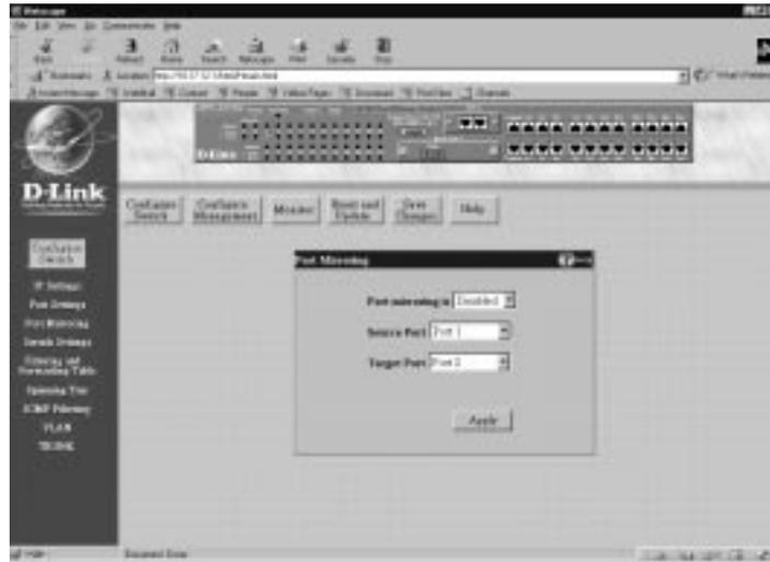
The Switch allows you to copy frames transmitted and received on a port and redirect the copies to another port. You can attach a monitoring device to the mirrored port, such as a sniffer or an RMON probe, to view details about the packets passing through the first port.
