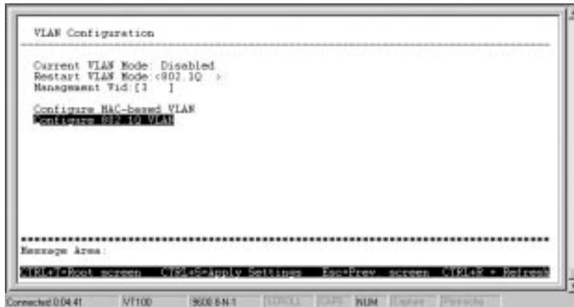
Figure 6-24. VLAN Configuration
