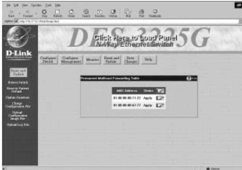
**Multicast filtering blocks or forwards traffic over each port for one multicast group. You can configure each port on the Switch to forward traffic for the specified multicast group.**
