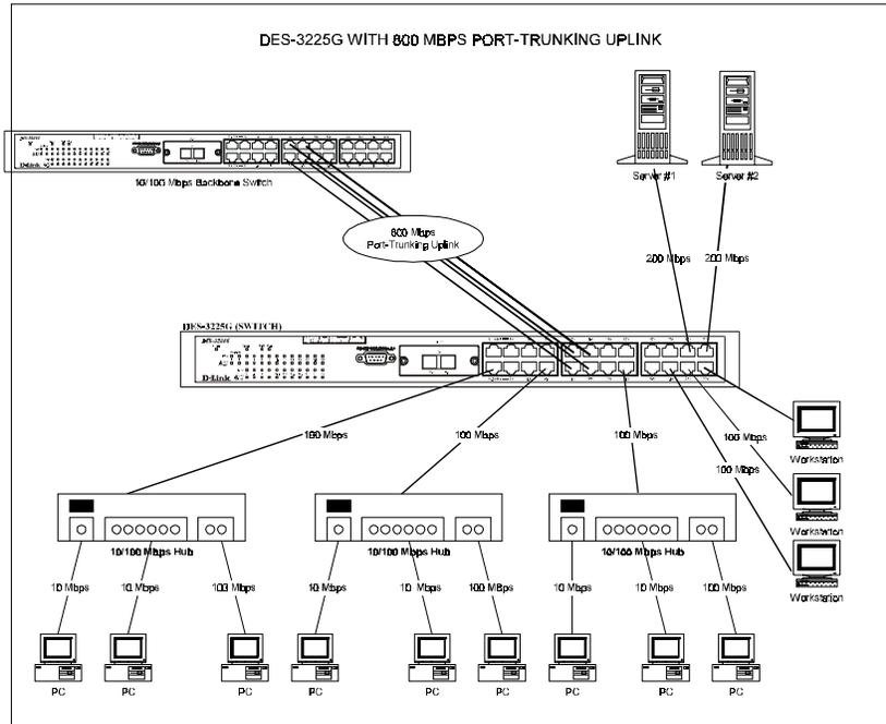
The switch treats all ports in a trunk group as a single port. As such, trunk ports will not be blocked by Spanning Tree.
