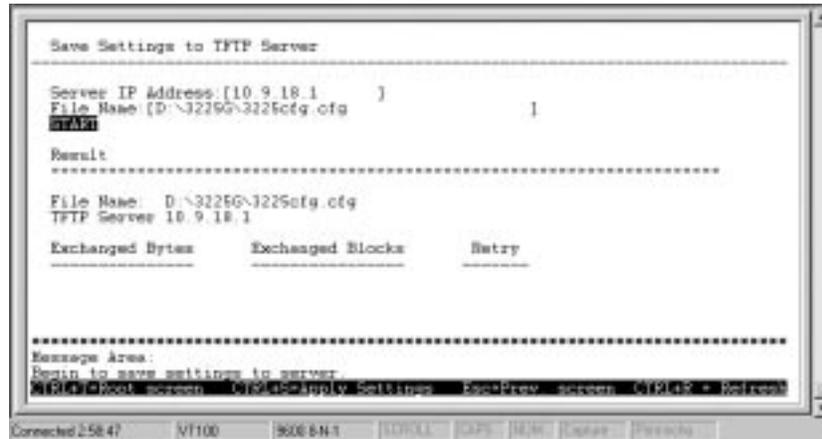
Figure 6-37. Upload Configuration File screen
