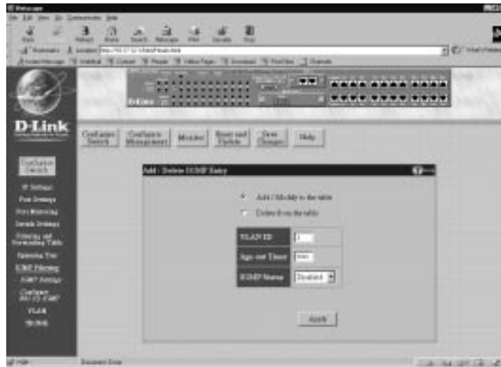
To Add/Modify to the table or Delete from the table, check the desired option button, enter a value from 1 to 2047 in the VLAN ID field, enter a value between 30 and 999 in the Age-out Timer field, enable or disable the IGMP Status control, and then click Apply.
