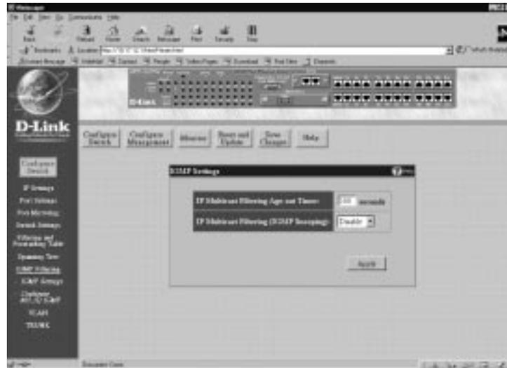
**Internet Group Management Protocol (IGMP) snooping allows the Switch to recognize IGMP queries and reports sent between network stations or devices and an IGMP host. When enabled for IGMP snooping, the Switch can open or close a port to a specific device based on IGMP messages passing through the switch.**
