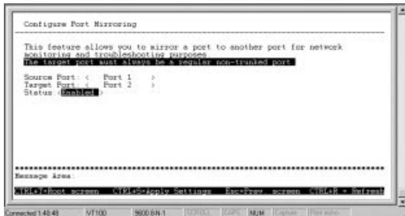
Figure 6-15. Configure Port Mirroring screen
