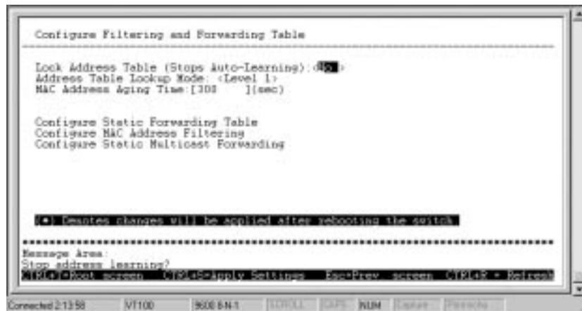
Figure 6-19. Configure Filtering and Forwarding table screen
