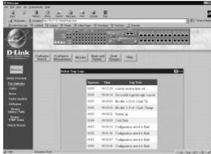
The Switch can send event information to its own logs, to designated SNMP trap receiving stations, and to the PC connected to the console manager. Clicking the Next Page hyperlink at the bottom of the screen will allow you to display the complete Switch Traps Log.
