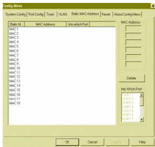
Figure 5.5 Screen shot of the static forwarding table of the Switch Configuration Software
