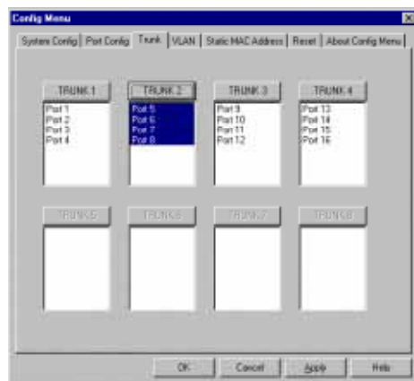
Figure 5.7 Screen shot of the trunk assignment menu of the Switch Configuration Software
