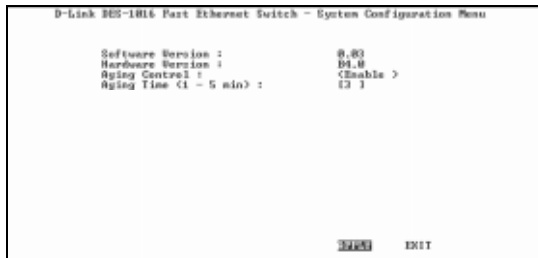
Figure 5.2 Screen shot of the configuration menu of the DOS Switch Configuration Software
