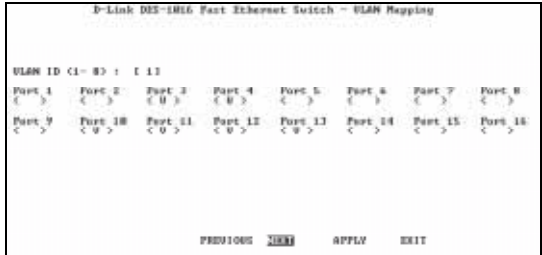
Figure 5.10 Screen shot of the VLAN configuration menu of the Switch Configuration Software
