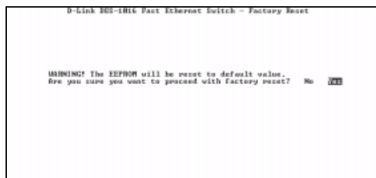
Figure 5.12 Screen shot of the system reset of the Switch Configuration Software
