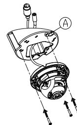
Remove the inner cover and adjust the angle and rotation of the camera as desired, then put the inner cover back in place.
