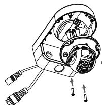
Remove the inner cover and adjust the angle and rotation of the camera as desired, then put the inner cover back in place.
