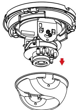
Loosen the adjustment screw on the side of the camera, then retighten it after moving the camera to the desired angle. You can also rotate the camera by grasping the camera and turning it left or right.
