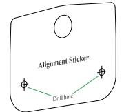
Use the provided screws to mount the DCS-37-1 to the wall.
