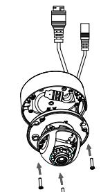
Remove the inner cover and adjust the angle and rotation of the camera as desired, then put the inner cover back in place.
