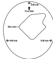
Use the provided screws to mount the DCS-37-3 to the wall using the inner mounting holes.
