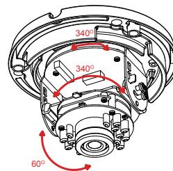
When you are done adjusting the camera's angle, put the inner cover back into place.
